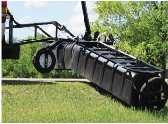
Roadside sprayers feature breakaway booms. The gauge wheels are located at the center and outer edge to ensure booms follow varying terrain.
